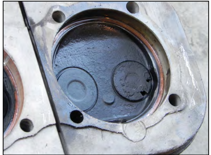
#5 Cylinder loaded with carbon and the burned out exhaust valve. See dark spots on right.
