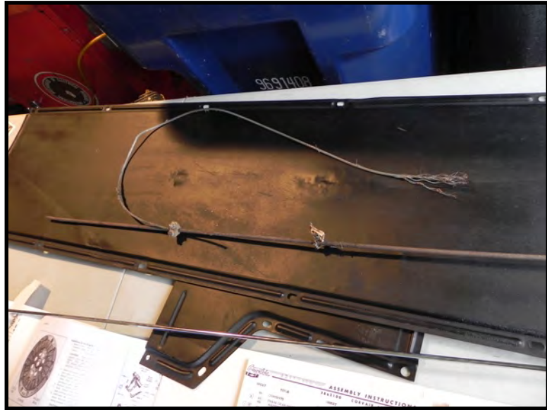
Broken cable above, and new replacement below. The broken cable was an emergency bolt on from a previous repair.
