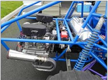
At this time I put in a 4 speed 091 VW bus trans. This is the strongest VW trans made. It is suppose to be almost as strong as a Corvair trans, but a lot lighter. Trans and trans axial are one piece aluminum. Rebuilt by Larry Harvey of Yuma. Another duner.
