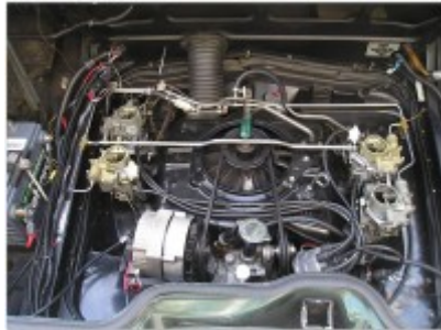
Figure 1- Rebuilt four carbs installed with new fuel lines. Note they lead in from front, as they lead from an electric fuel pump.
