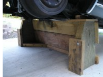
Figure 2 - Ron's stand to support the back of the car is high enough to drop the drive train out and clear everything. It is placed just in front of the drive train, and across the normal jacking pads.
