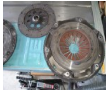
Figure 6 - Old clutch disc and pressure plate showing the worn hot spots on the face.
