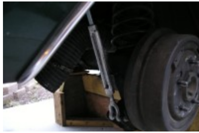
Figure 3 - Ron's heavy turnbuckles to replace the shock absorbers and adjust the wheel height to relieve stress while removing and replacing bolts for the strut rod.
