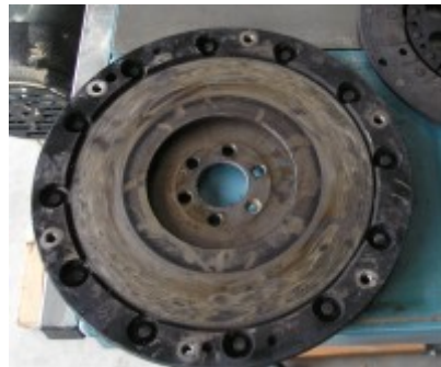
Figure 5 - Old flywheel showing worn and hot spots on the face.
