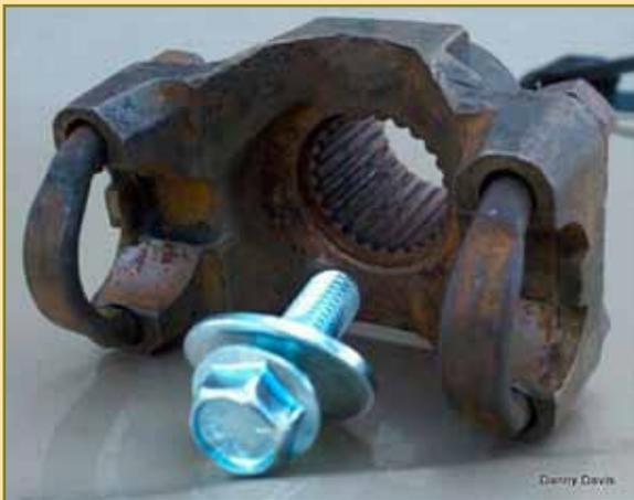
Above is the replacement yoke along with an example of the retaining bolt and washer. This bolt has a serrated flange head that serves as a lock. I also use Loctite on the threads, You don't want this part coming loose!! It's actually an easy repair, but one of those that would be better done before it comes apart!
