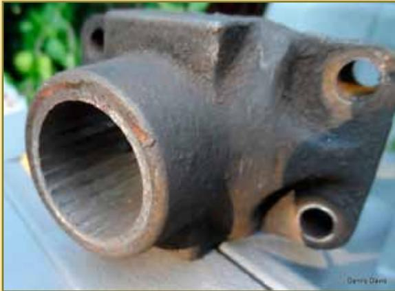
This is what results from a loose joint. The yoke is cast iron and the internal splines are easily chewed up by the much harder steel of the axle splines.
