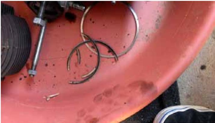
**BROKEN RINGS** – will usually cause smoke out of the tailpipe. The same with bad guides. While it is possible that a blocked vent system can cause excessive pressure, this is easy to rule out by cleaning out the draft tube or pcv tube. Nearly all cases of excessive internal pressure will require at least removing the head of the offending side - remember that if you
